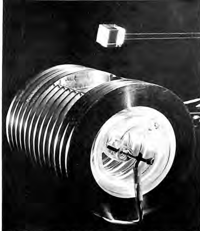
RUBY CRYSTAL, the heart of a new scientific breakthrough device called a laser.
