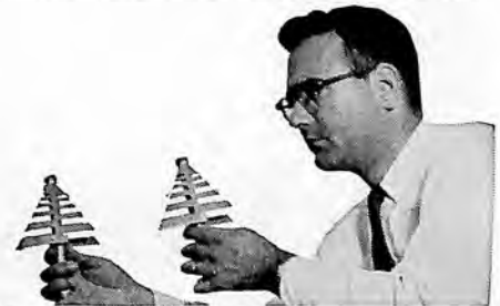
ESAR contains nearly 9,000 of these Christmas tree type antennas. "Electronically steerable," they can watch thousands of missiles, aircraft, and satellites simultaneously.
