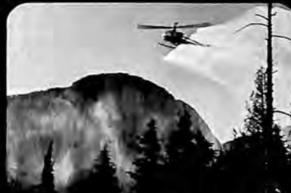
El. 10,000 ft. Two 12 E's fly 80 gal. sprayloads; 60 flights in 4 hrs.
