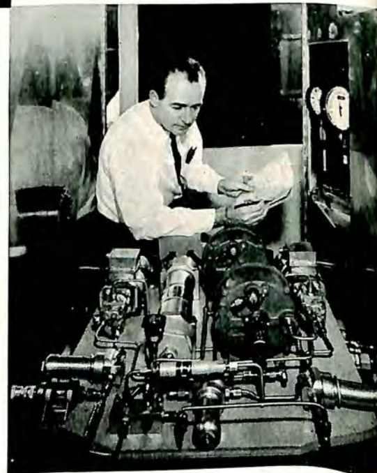
Advanced type of primary and emergency fluid power supply system developed and built by Vickers being readied for feasibility test in an environmental chamber.
