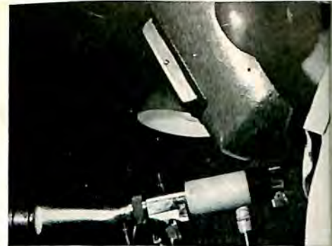
Extremely high temperature material problems encountered on re-entry into earth's atmosphere are studied with the aid of a plasma jet capable of 30,000°F.
