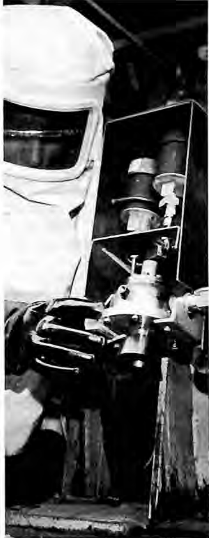
TECHNICIANS ready new missile reaction control unit.
