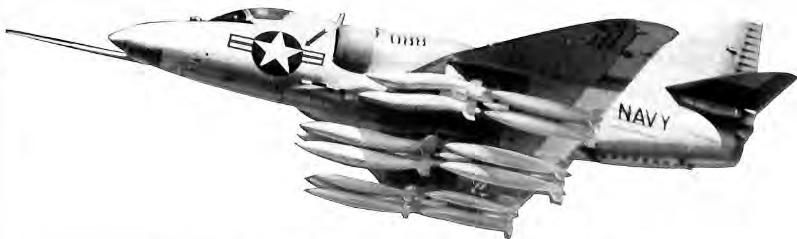
NEW BOMB RACK adapter for Navy A4D increased bomb load six times.
